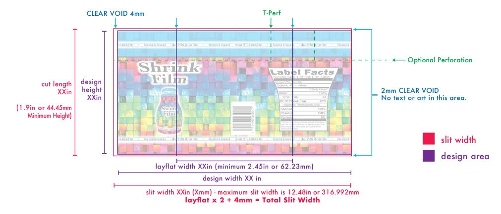
• Slit width: The total width of a shrink sleeve before it is seamed.
